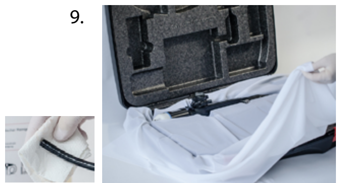
9. For transportation store your scope within a protection cloth or film. Use a cotton tissue gaze for the distal tip of the endoscope to collect rest water
