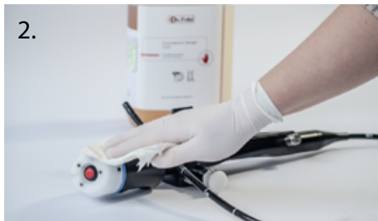
2. Clean scope outside with damp cloth and cleaner (Dr. Fritz enzym cleaner FLEX), diluted as instructed, moisten.
